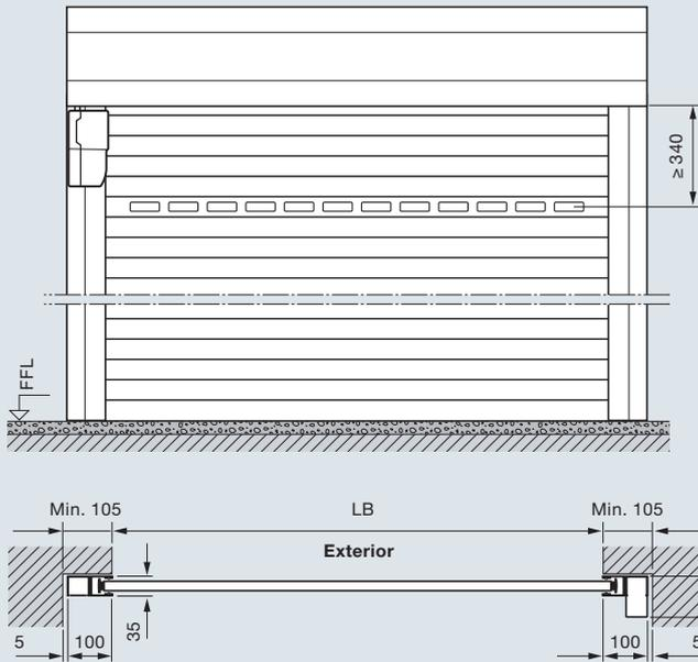
Internal roller garage door: Fitting in the opening, interior view
